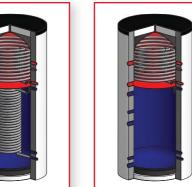
With a separating metal sheet and 1 stainless-steel heat exchanger
